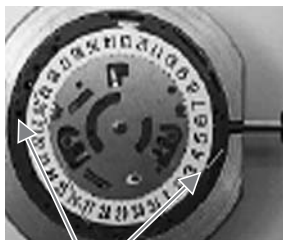
Positions of the slots on the main plate (two positions)
